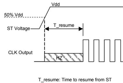
Figure 5. Standby Resume Timing ( $\overline{ST}$  Mode Only)
