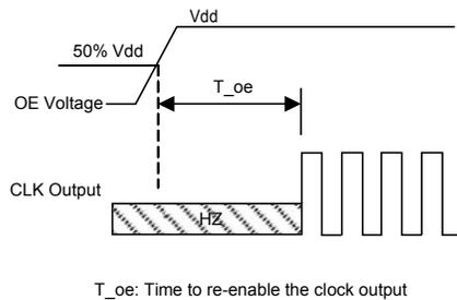
Figure 6. OE Enable Timing (OE Mode Only)
