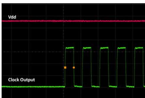
**Figure 18. Startup Waveform vs. Vdd
