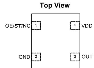
**Figure 1. Pin Assignments**
