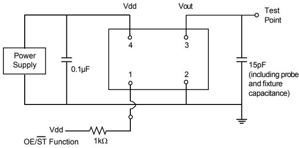
**Figure 2. Test Circuit**
