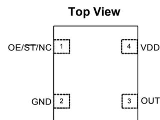
**Figure 1. Pin Assignments**
