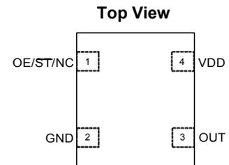
**Figure 1. Pin Assignments**
