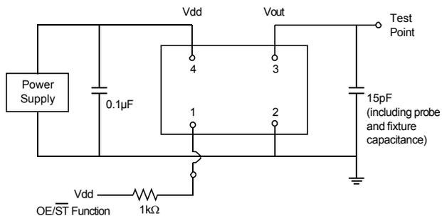
**Figure 2. Test Circuit**
