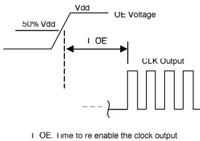
Figure 6. OE Enable Timing (OE Mode Only)
