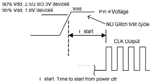
Figure 5. Startup Timing (OE/ $\overline{ST}$  Mode)
