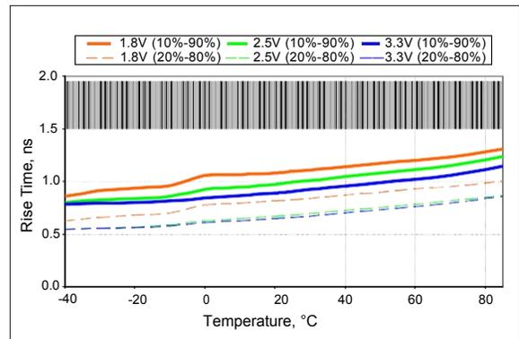
Figure 13. Rise Time vs Temperature, 100 MHz Output
