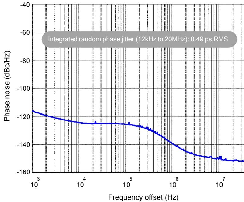
Figure 2. Phase Noise, 156.25 MHz, 3.3V, LVC MOS Output
