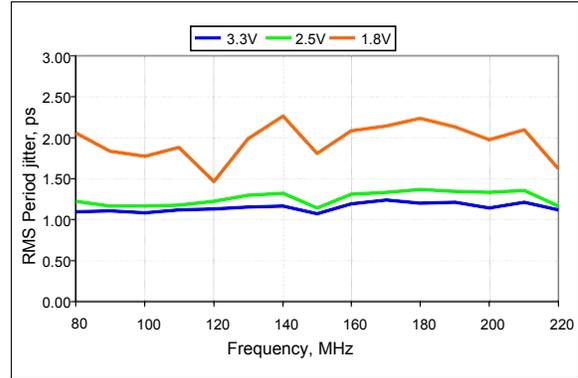
Figure 9. RMS Period Jitter vs Frequency
