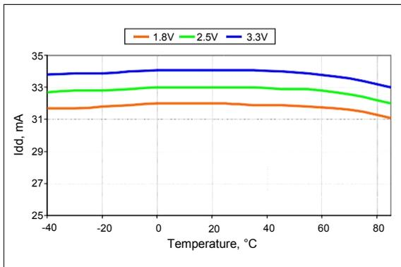
Figure 12. Idd vs Temperature, 100 MHz Output
