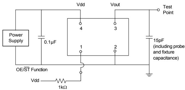
Figure 3. Test Circuit
