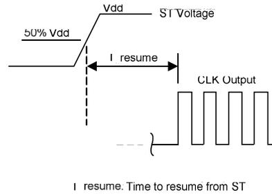
Figure 6. Standby Resume Timing ( $\overline{ST}$  Mode Only)
