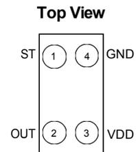
**Figure 1. Pin Assignments**
