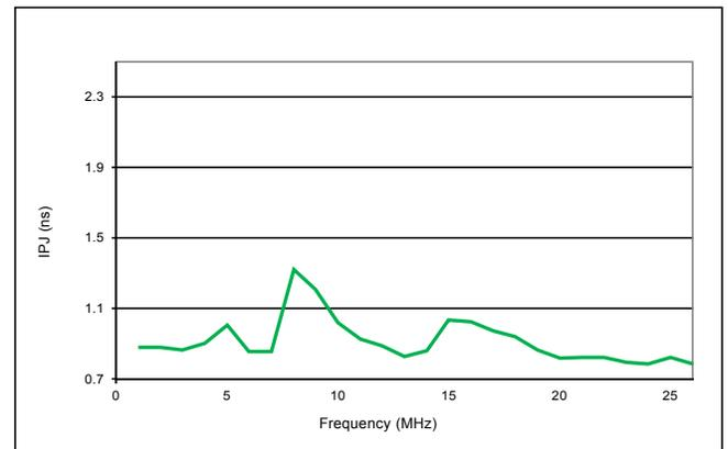
Figure 13. RMS Phase Jitter Random vs Frequency<sup>[8]</sup>
