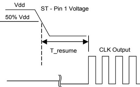
$T_{resume}$ : Time to valid clock output from the time ST pin crosses 50% threshold
