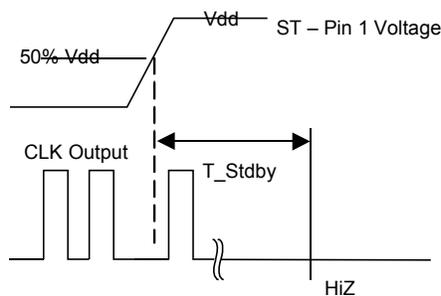
$T_{Stdbby}$ : Time for output to go high-Z from the time ST pin crosses 50% threshold
