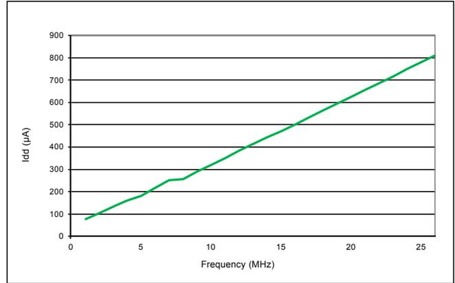
Figure 9. I<sub>dd</sub> vs Frequency with 10pF load
