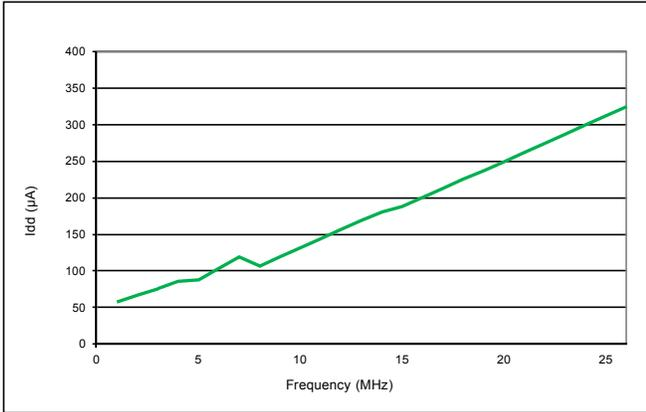
Figure 8. I<sub>dd</sub> vs Frequency without load
