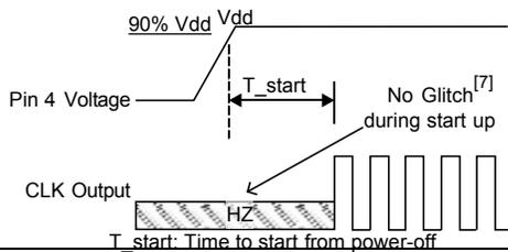
Figure 4. Startup Timing (OE/ ST Mode)
