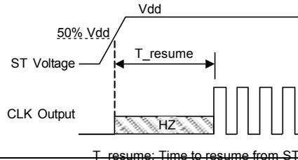
Figure 5. Standby Resume Timing ( ST Mode Only)
