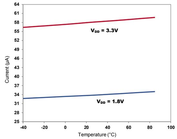
Figure 12. Supply Current vs Temperature (F<sub>OUT</sub> = 2 MHz)
