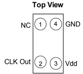
**Figure 1. Pin Assignment**
