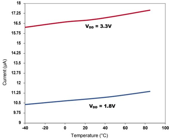
Figure 9. Supply Current vs Temperature (F<sub>OUT</sub> = 500 kHz)
