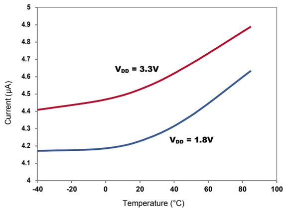
Figure 7. Supply Current vs Temperature ( $F_{OUT} = 100\text{ Hz}$ )
