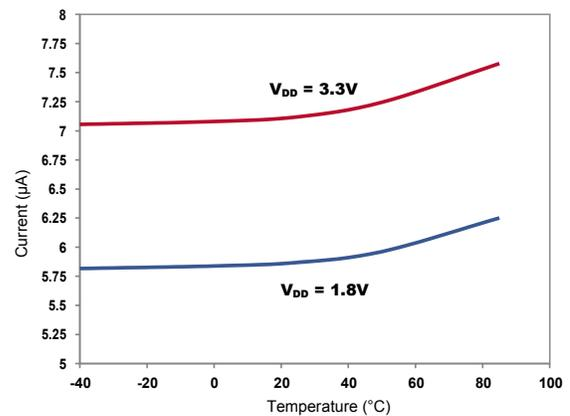
Figure 8. Supply Current vs Temperature ( $F_{OUT} = 100\text{ kHz}$ )
