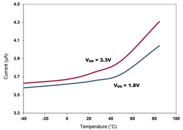
Figure 6. Supply Current vs Temperature ( $F_{OUT} = 1\text{ Hz}$ )
