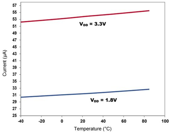
Figure 11. Supply Current vs Temperature (F<sub>OUT</sub> = 1.85 MHz)
