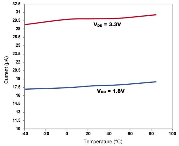
Figure 10. Supply Current vs Temperature (F<sub>OUT</sub> = 1 MHz)
