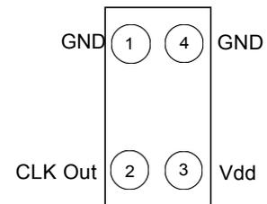
**Figure 1. Pin Assignments**
