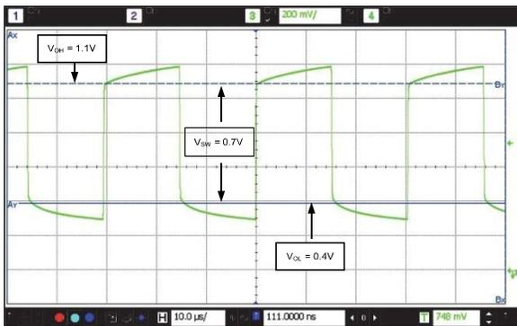
**Figure 4. JYJE1532AI-J4-D14-32.768 Output Waveform (10 pF load)**
