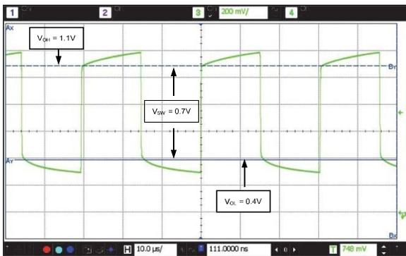
Figure 12. NanoDrive™ Output Waveform
