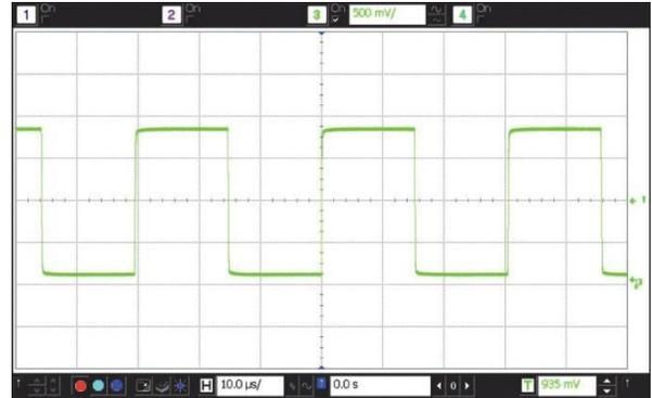
**Figure 5. LVCMOS Waveform (Vdd = 1.8V) into 15 pF Load**
