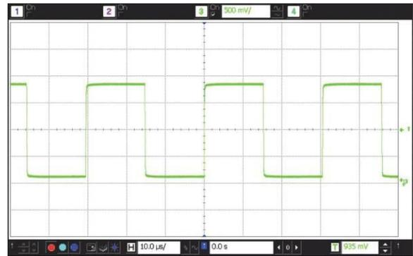
Figure 13. LVC MOS Output Waveform
