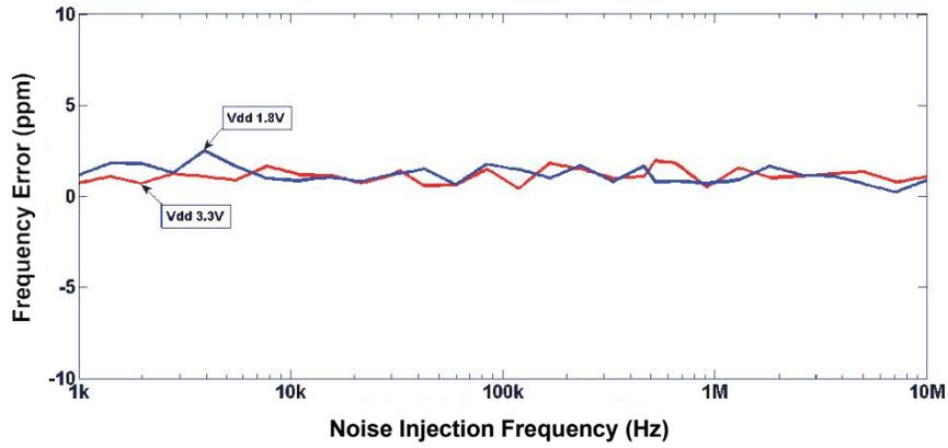
Figure 11. Power Supply Noise Rejection
